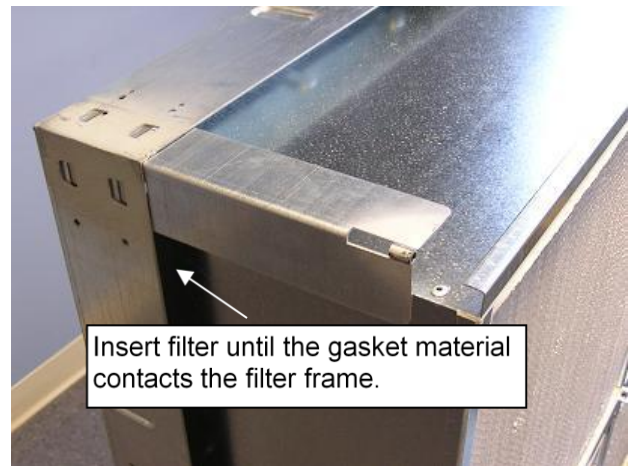
Figure 4: Insert HEPA filter into frame, until the gasket comes in contact with the holding frame.
