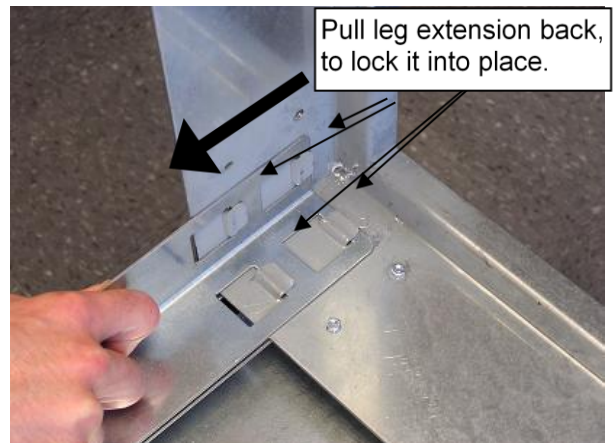
Figure 2: Place leg extension over the frame tabs, then pull back to lock the leg extension into place.
