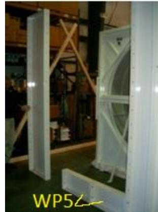
7.12. Seal each joint between the panels ON THE EXTERIOR SEAM ONLY with the Sealer/Caulking provided including between the Plenum Wall and Flashing Panel. Seal/Caulk both inside and outside seams. Most enclosures operate under a negative/vacuum so the outside seal is the most important.
