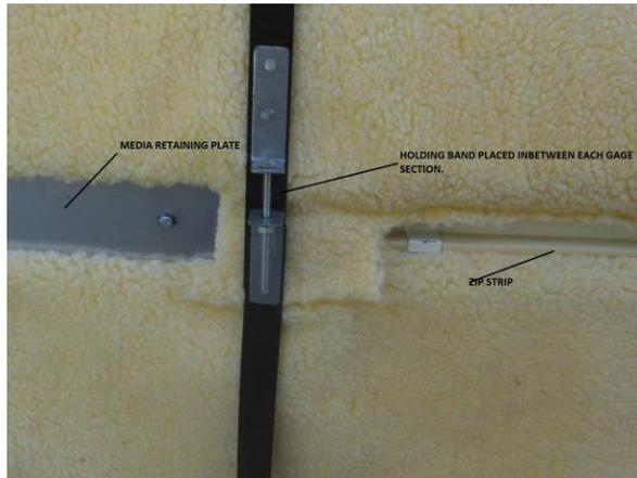
**NOTE:** Check the band alignment by rotating the cages and inspecting closely to see if bands stay true.
