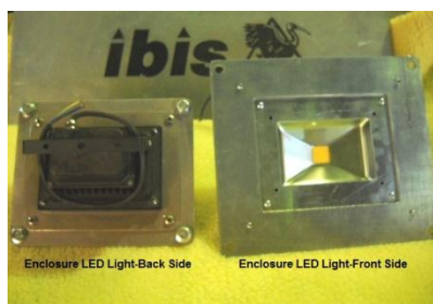
Exterior LED Light Fixture
